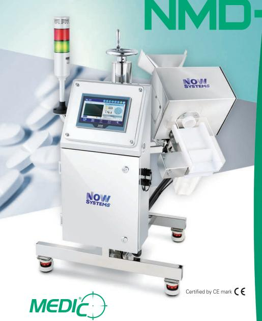
**NMD530 Series(MEDIC)** Pharmaceutical type metal detector is the most delicate system among NMD530 Series range products. Offering unparalleled accuracy in the detection of metallic contaminants in pharmaceutical products, it can detect and reject microscopic particles in pharmaceutical production lines at speeds of up to 15,000 tablets per minute. Even in difficult application, our innovative technology continues to provide exceptional performance.
